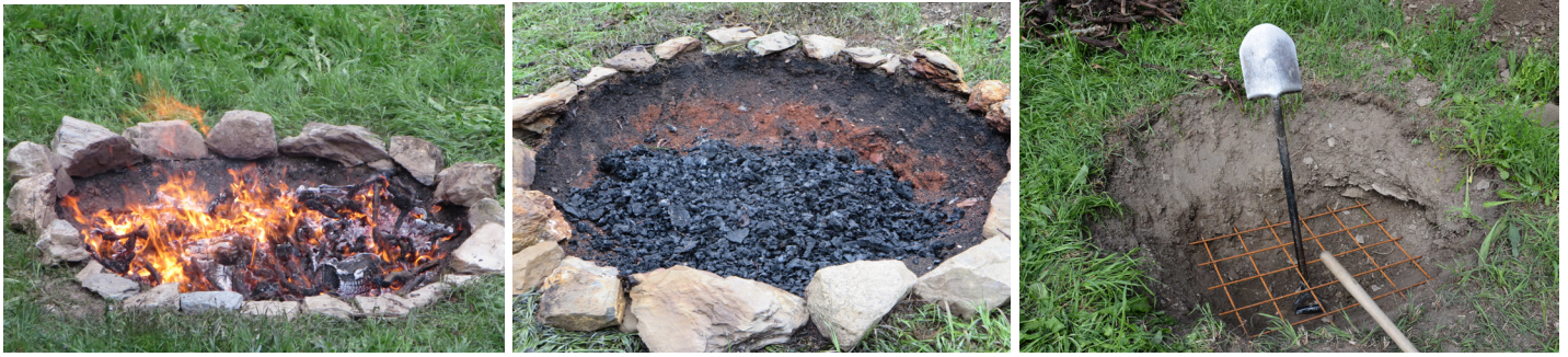
Fig. 6: Production of biochar in a 90 cm deep pit with a stone rim (Images: Ithaka-Institute).
