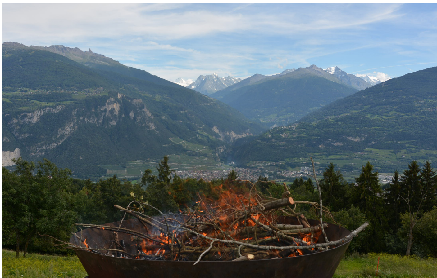
Fig. 9: Once a strong ember bed brings the pyrolysis temperature up to 700 ° C, fresh wood can be added. The Kon-Tiki functions as both a feedstock dryer and a pyrolyzer.
