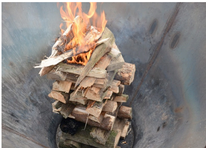
Fig. 10: igniting the wood chimney in the middle of the Kon-Tiki.
