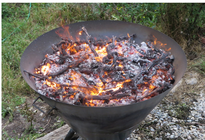
Fig. 11: When the top layer of biomass begins to coat with ash, it is the right time to add the next fuel layer. The biomass becomes completely charred then in the lower layers.
