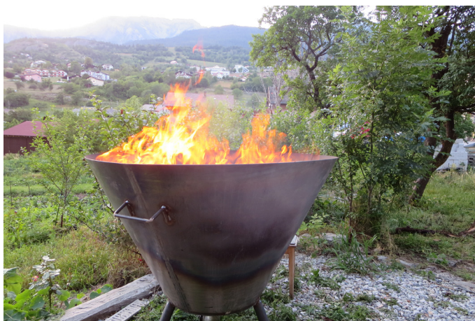
Fig. 7: The first Kon-Tiki had a diameter of 150 cm, a height of 90 cm and a capacity of 850 liters. It was built by Markus Koller.
